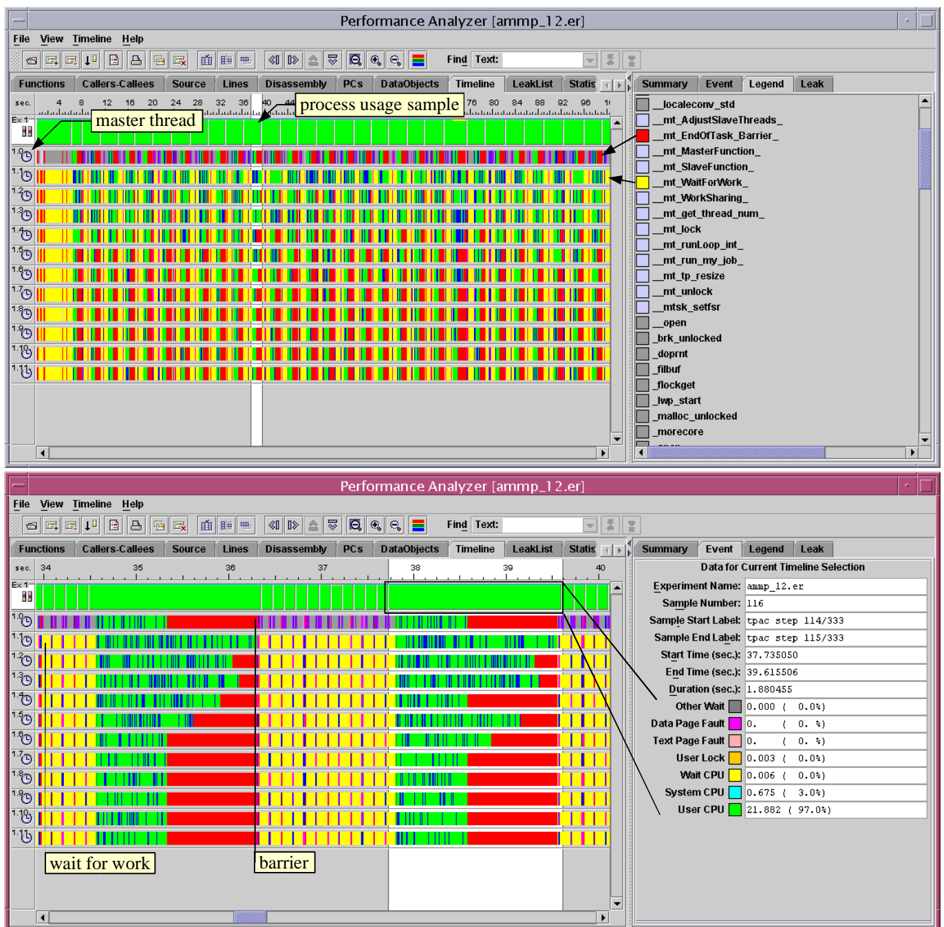
Figure 11: Timeline views showing full experiment duration and zoomed with tpac step 114/333 selected
